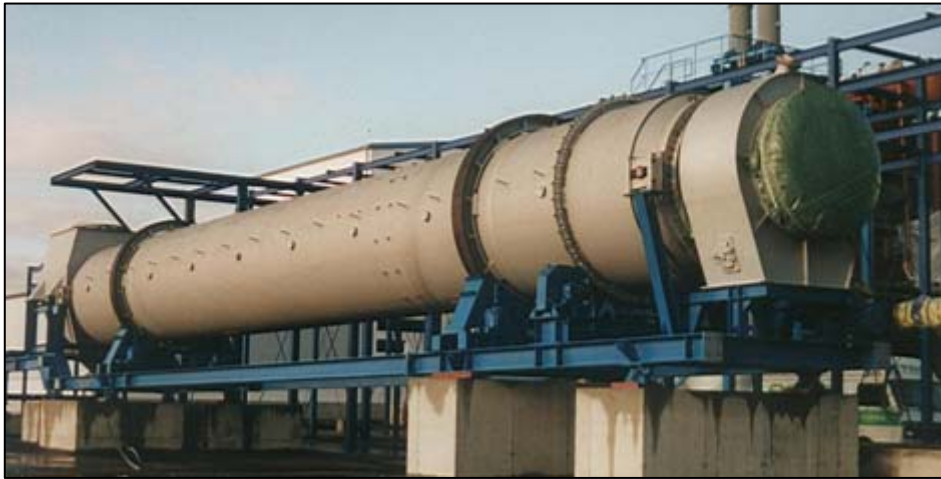
Picture D.1 appearance for biomass pyrolysis furnace made completed
